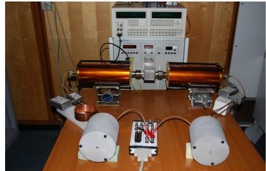
Basic circuit of the phase comparator.  $SH_1$  and  $SH_2$  denote the two shunts being compared. Two active guarded transformers (AGTs) are employed as wideband decoupled precision transmitters.
